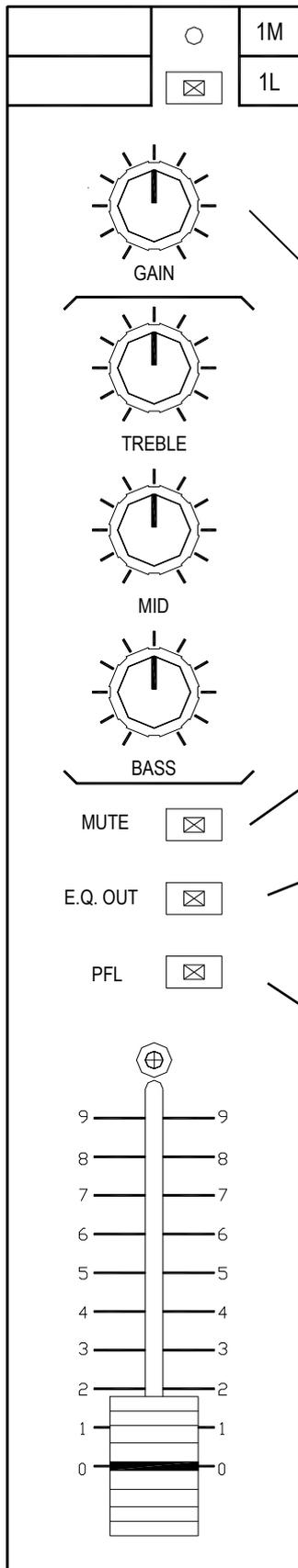
Input selector switch selects input used. M = microphone (XLR connector). L = stereo line (phono connectors). 2 parallel pairs of phono sockets allow easy parallel of source to a second input if required.
