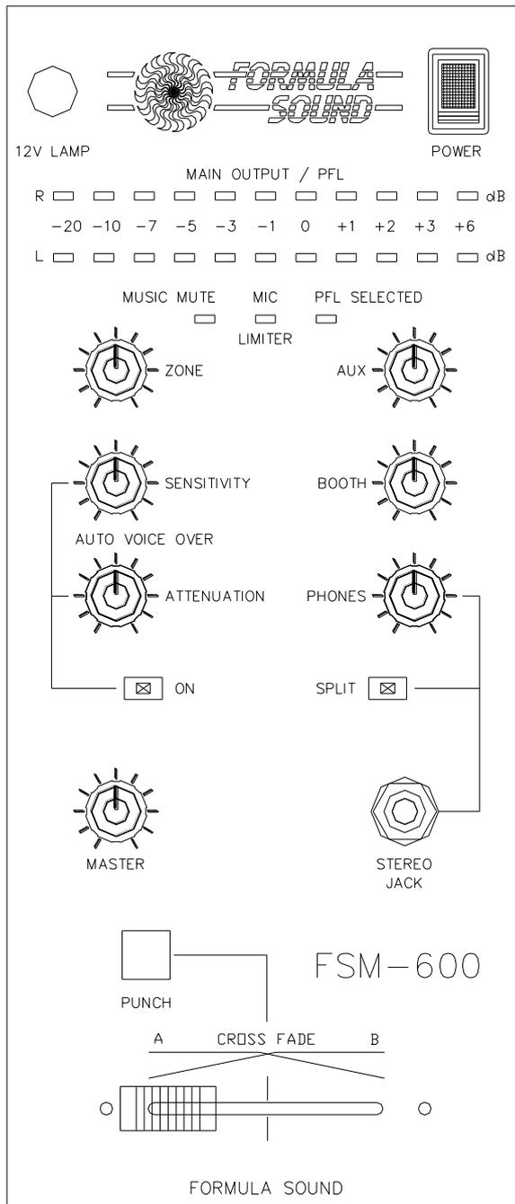
Power switch switches the mains feed to the mixer power supply. N.B. to avoid switch on thrumps audio systems need powering up in sequence. A good rule to remember is - power amps on last and off first.
